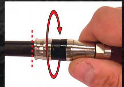
Insert cable into connector push firmly while rotating clockwise until the connector reaches the mark on the jacket.
