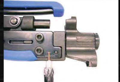
Ensure cable is prepared to 1/4" x 1/4" dimensions
