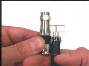
Mark cable at the base of the connector with thumbnail or other marking device
