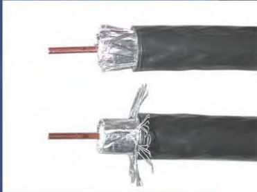
Ensure there is no dielectric, braid or foil wrapped around center conductor. Fold back braid.
