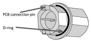
To ensure potential corrosion over a long period of time have no effect on the electrical performance, the outershield of the F-connector is soldered directly onto the printed circiut board (PCB). Normally the outer shield of the F-connector is soldered to the housing and from there connected to the PCB, but as the housing can be more vulnerable to electrolytical corrosion as its made from zinc and
